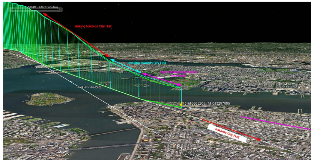
Figure 21: Estimation of UA175 route derived from analysis of multiple films and the NTSB Radar Data Impact Speed Study. White lines indicate headings flown at different parts of the route (Kobs, 2025).
