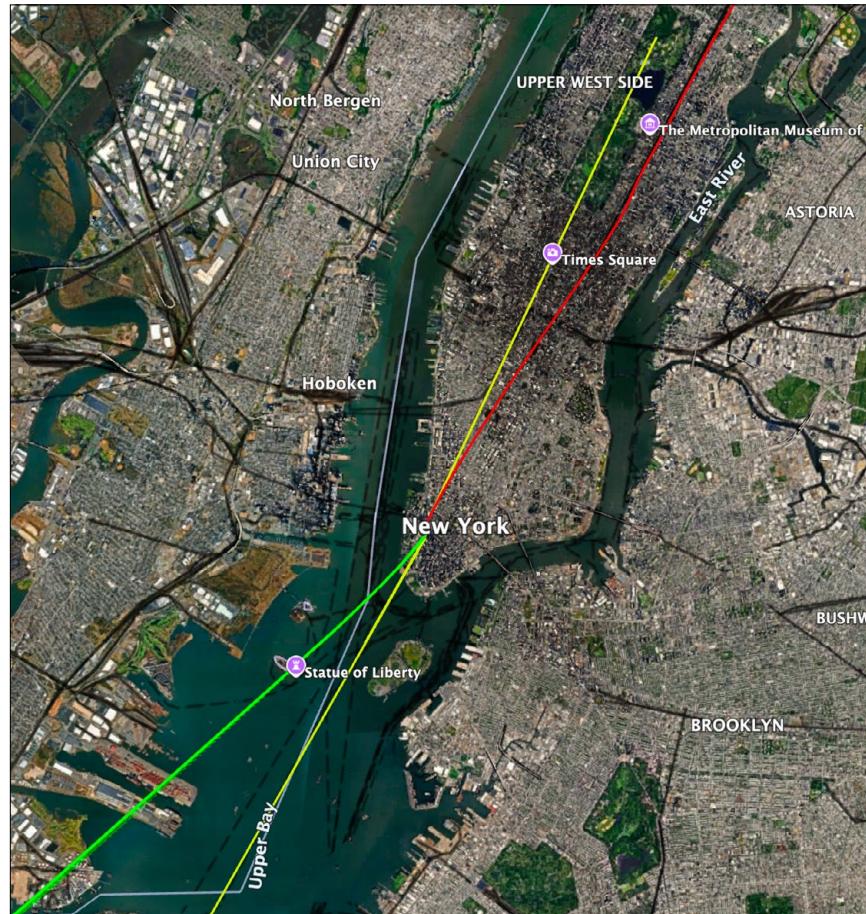
Figure 29: Estimation of reported flight tracks using Google Earth (with UA175 in green and AA11 in red). Yellow lines show approximation of tracks running perpendicular to the building faces.
