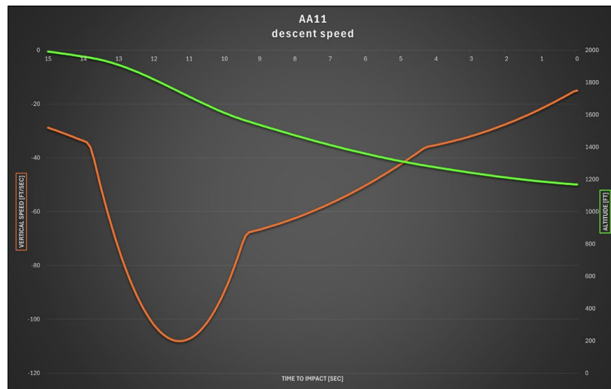
Figure 25: Estimation of vertical speed rate of descent changes during the last 15 seconds of flight (Kobs, 2026). Derived from analysis of NTSB Radar Data Impact Speed Study (2002c).
