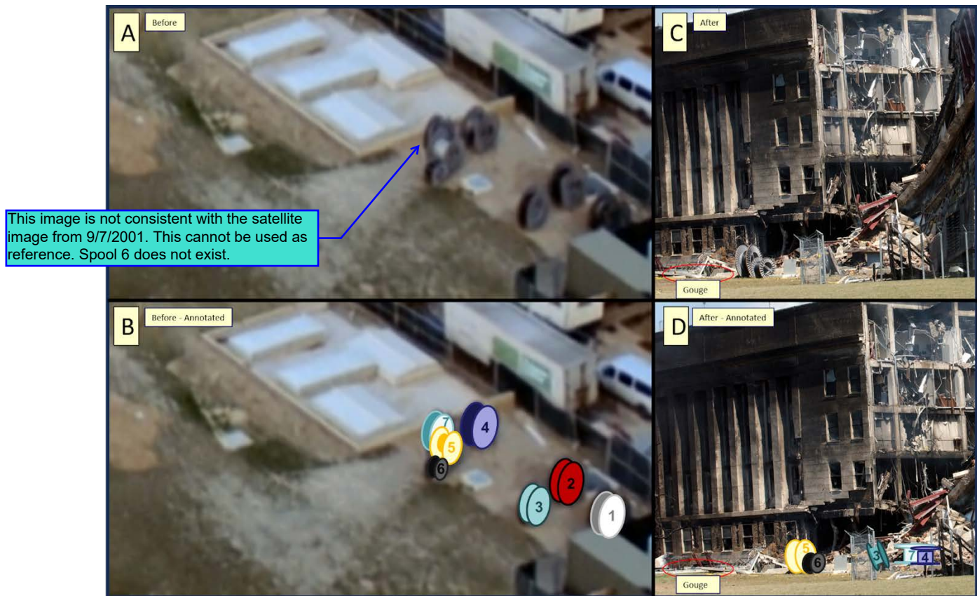
Figure 12: Location of wire spools before and after impact.
