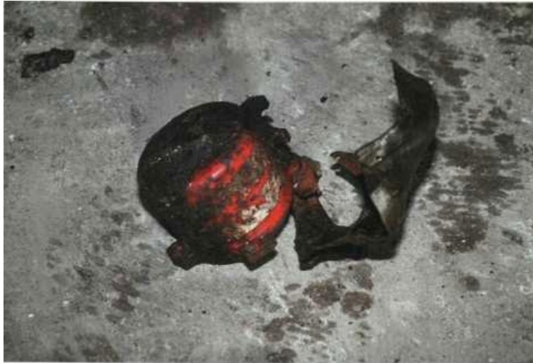
Figure 14 Memory module of Flight Data Recorder (FDR) found in the Pentagon. The data found on this memory module will be discussed in a separate paper yet to come.
