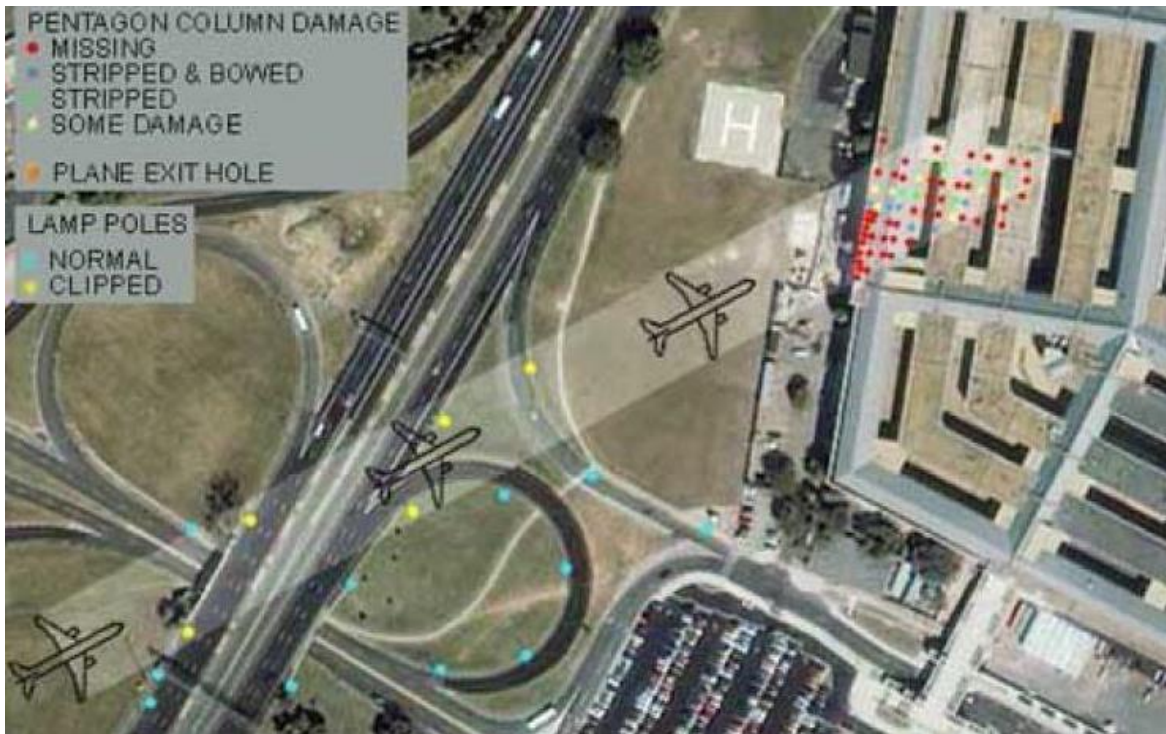
Figure 1 Alignment of light pole damage with interior damage in the Pentagon.
