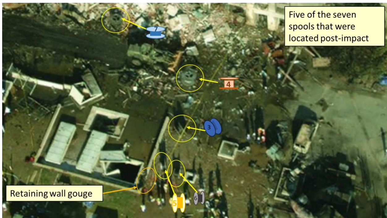
Figure 13: Overhead view of the location of the wire spools after the impact.
