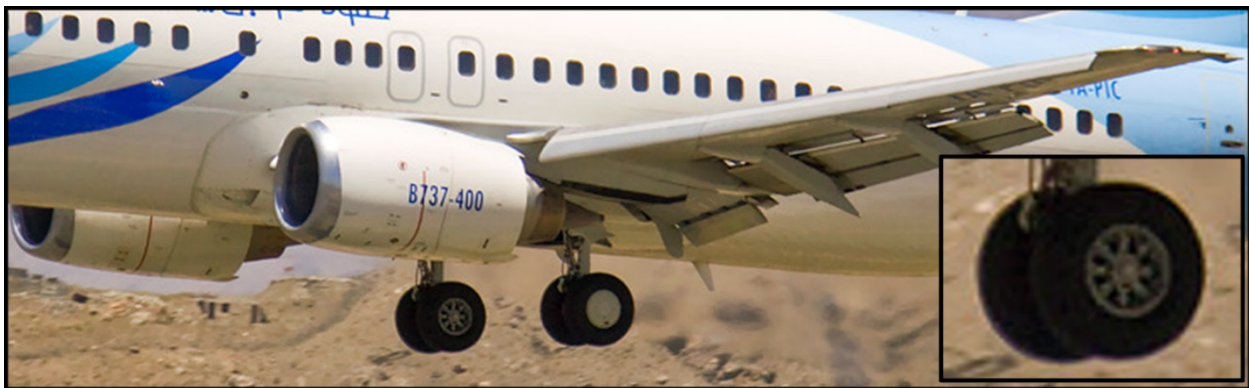
Figure 24: Wheelsets of a Boeing 737-400 showing different inner and outer hub designs with wedge-shaped cut-outs.
