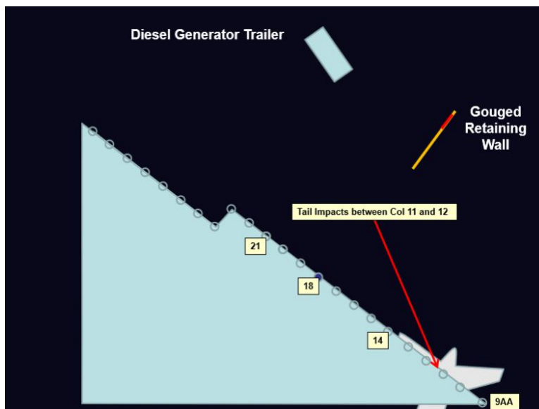
Figure 11: Yaw rotation causes tail section to impact between columns 11 and 12
