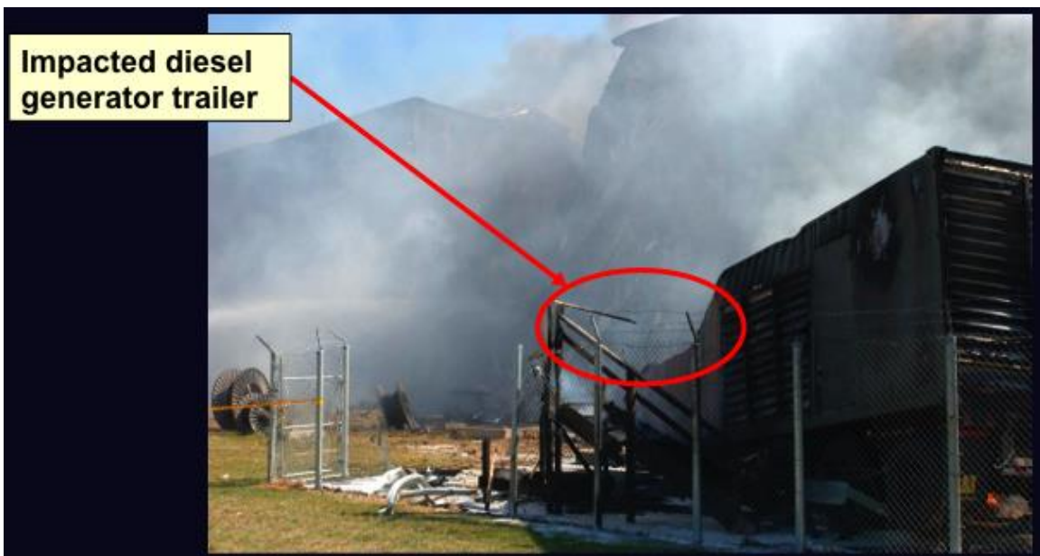
Figure 19: The generator trailer was gouged and rotated toward the Pentagon. This impact caused the plane to roll to the left and rotate around a vertical axis.
