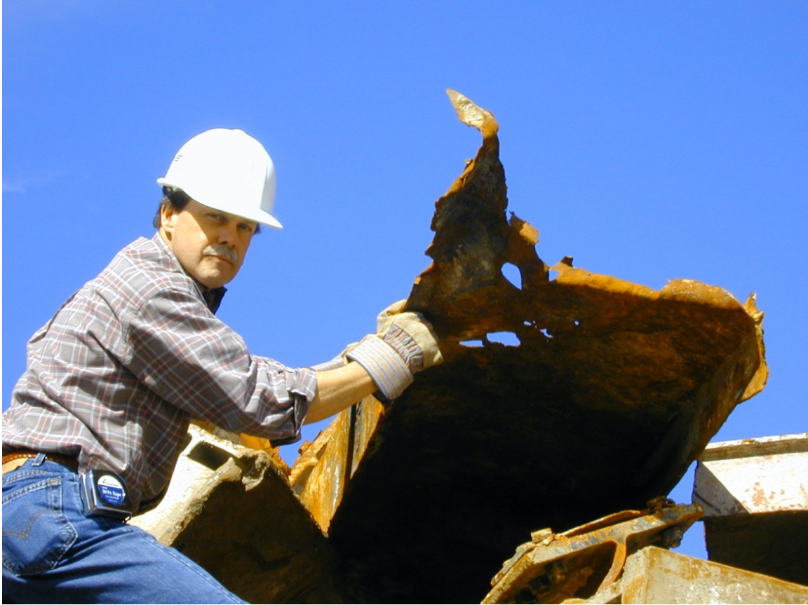
Figure 17: NIST’s John Gross next to the severely eroded WTC 7 steel member during the FEMA investigation.
