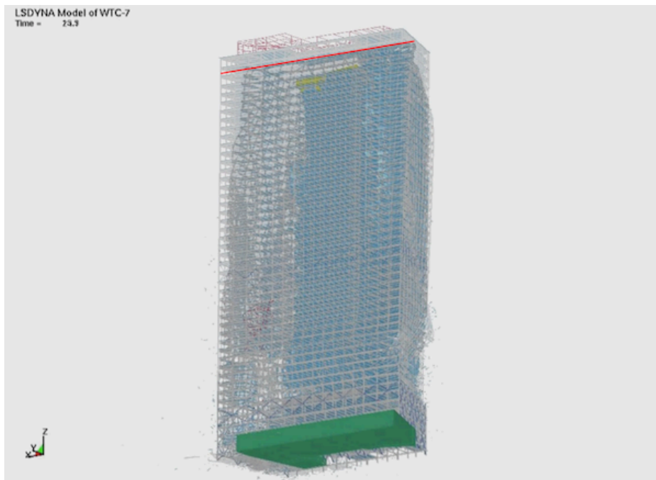
Figure 10: Roofline in NIST’s global collapse analysis descends ~1.5 stories (~6 meters) in 1.8 seconds.
