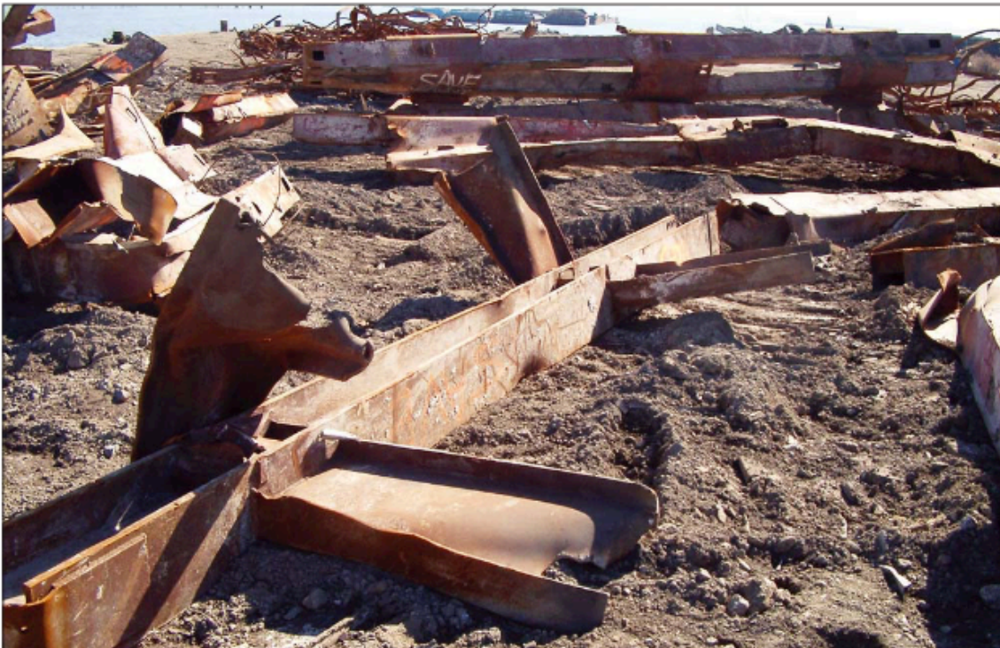
Figure D-14 WTC 7 W14 column tree with beams attached to two floors.
