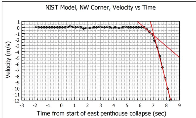
Figure 13: Vertical velocity vs. time for the northwest corner. Transitional acceleration =  $-1.85 \text{ m/s}^2$ . Final acceleration =  $-8.38 \text{ m/s}^2$ .
