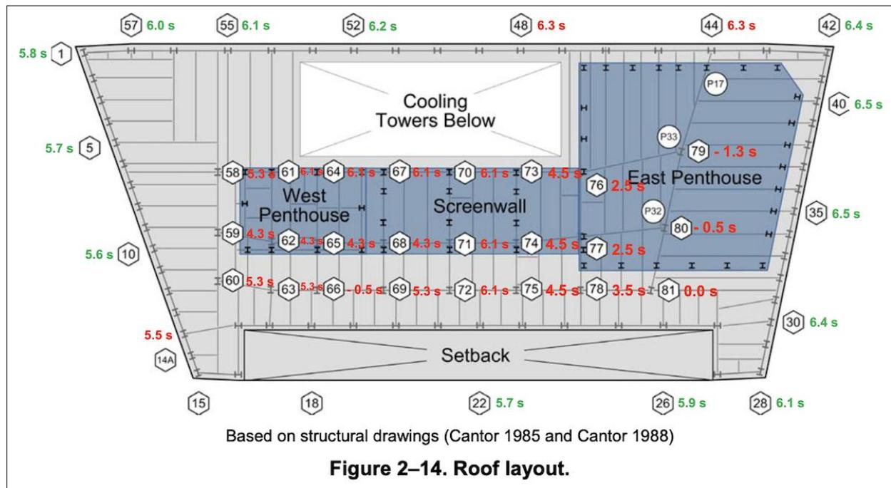
Figure 6: The timing of NIST’s column failure sequence. 0.0 is the start of the east penthouse collapse.
