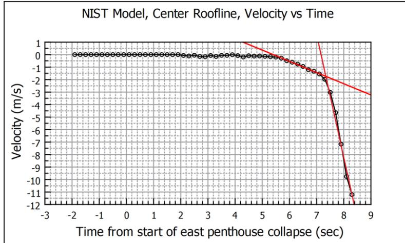
Figure 11: Vertical velocity vs. time for the east center roofline. Transitional acceleration =  $-0.898 \text{ m/s}^2$ . Final acceleration =  $-8.70 \text{ m/s}^2$ .
