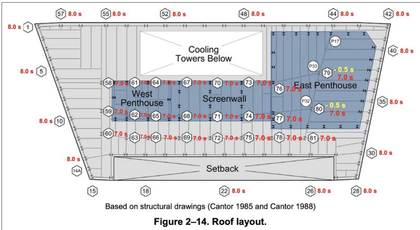
Figure 14: Hypothesized column failure sequence with estimated approximate failure times. Yellow indicates column failures high in the building. Red indicates column failures low in the building.
