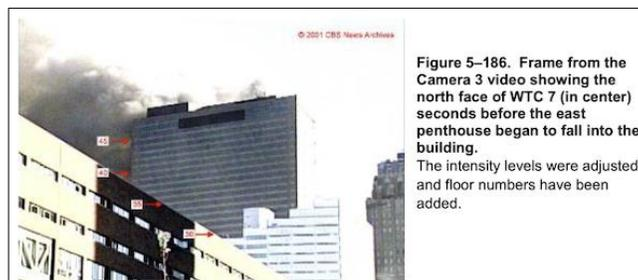
“To obtain a better understanding of the vertical motion of the building in the first several seconds of descent, the motion of the north face was studied in more detail **by tracking the vertical position of a point near the center of the roofline** using the same video. . . .
