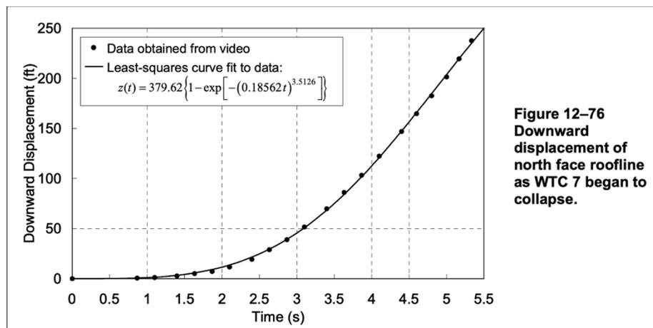
“As noted above, the collapse time was approximately 40 percent longer than that of free fall for the first 18 stories of descent. **The detailed analysis shows that this increase in time is due primarily to Stage 1, in which column buckling was just beginning and gradual increases in displacement and velocity were observed. The three stages of collapse progression described above are consistent with the results of the global collapse analyses discussed earlier in this chapter.**”
