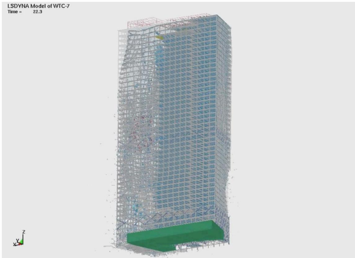
Figure 7: NIST’s global collapse animation at 6.3 seconds after the start of the east penthouse collapse laid over the animation at 0.1 seconds before the start of the east penthouse collapse.
