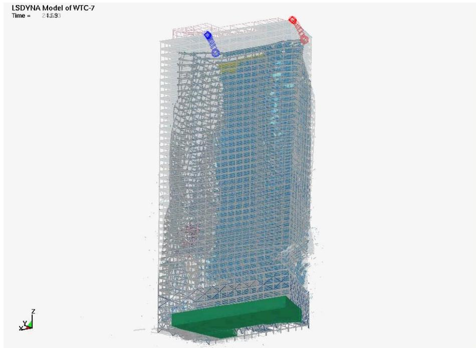
Figure 8: The final frame of NIST's global collapse animation, at 8.6 seconds after the start of the east penthouse collapse, laid over the animation at 0.1 seconds before the start of the east penthouse collapse. Blue dots track the motion at the east center roofline point. Red dots track the motion of the northwest corner.
