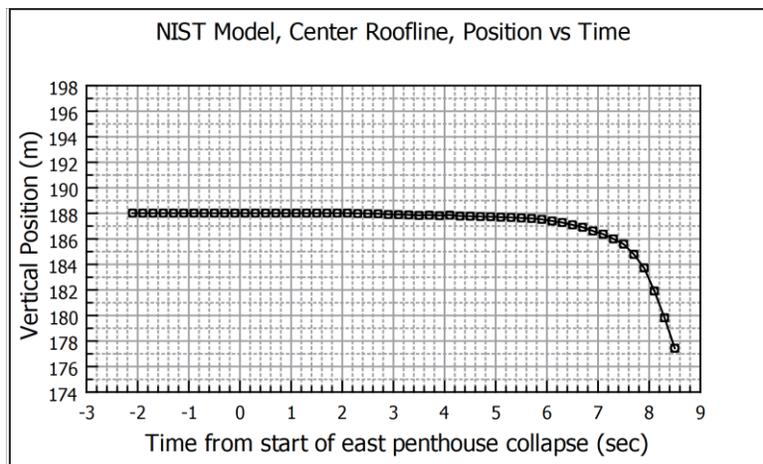
Figure 10: Vertical position vs. time for the east center roofline.
