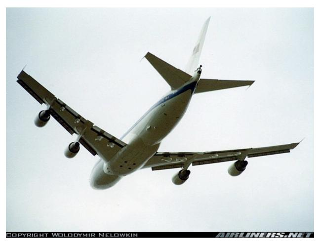
The spot is the only place on the 747 fuselage where the E-4B's otherwise conspicuous blue stripes are visible, from beneath. This establishes a positive ID, as no other airplane has this unique combination of features.
