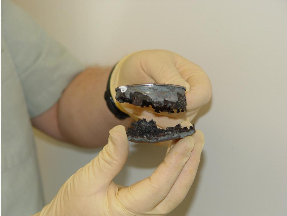
Above: in a fraction of a second, thermate cuts horizontally through a steel cup. Notice the high-temperature corrosion which occurred.
